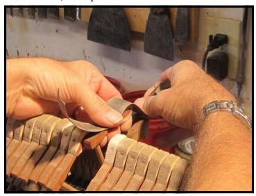
Hammers being filed to remove cut marks.
